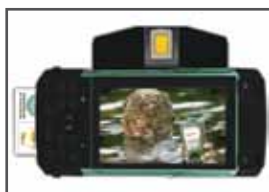
5" LCD, touchscreen, 1.6GHz CPU, 3 integrated scanners + CAC reader
