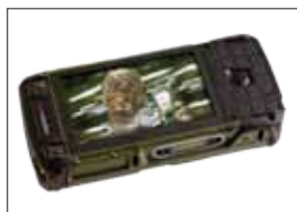
Opentec RPT 5 5" LCD, touchscreen, 1.6GHz CPU
