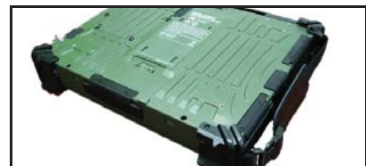
Rugged IP54 Magnesium alloy case
